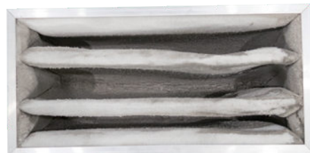
The filter that needs to be replaced
