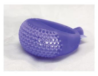
9. Remove the model from the mesh basket in dissolved solvent III for 20 seconds.
